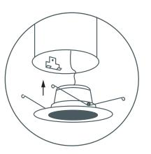
**2. Housing without torsion bracket.** Check that the "flip clips" are firmly attached. Center the fixture in the housing opening and gently push up until flush with the ceiling.
