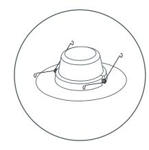
**2. Housing without torsion bracket.** Replace the torsion springs with the flip clips included in the packaging using a screwdriver.
