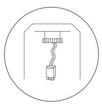
2. If it's a connector inside the housing, mate the connector with the terminal on the fixture directly.
