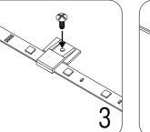
For suitable surfaces, provided clips and screws can be used to secure the strip in place. Do not reposition strip light once it is mounted.
